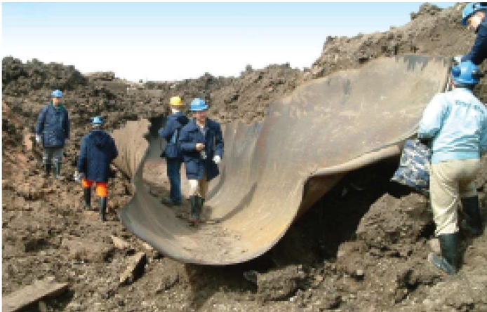
A running fracture – result of a test
